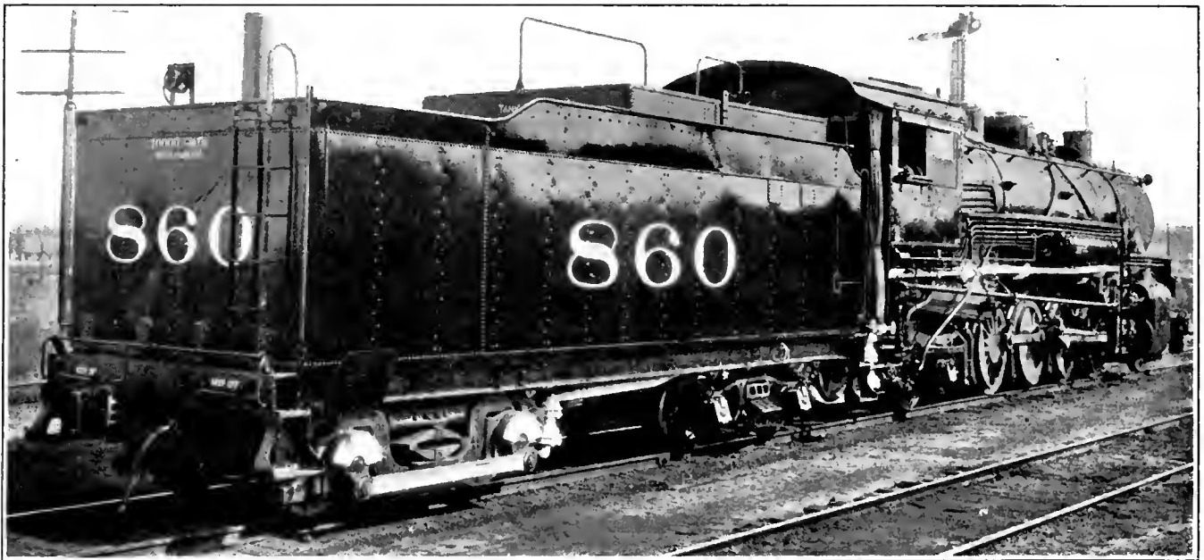
Locomotive Tender Equipped with Auxiliary Locomotive or Booster That Is Fitted with S K F Roller Bearings and Manufactured by the Bethlehem Steel Company
